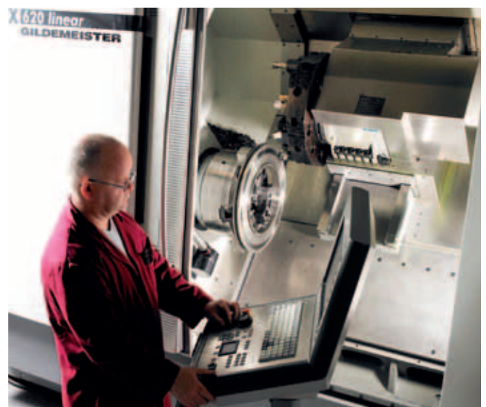
CAD/CAM machining of customised mould tools for Walkersele® production
